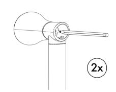
Drill 1/4" hole in marked locations. If drilling into tile, be sure to use a drill bit designated for tile. If mounting directly into stud or wood wall, secure lower end bracket to wall with mounting screws without drilling holes.
